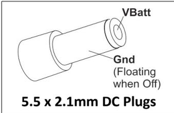
The front and rear power ports use 5.5 x 2.1mm DC jacks and present full battery voltage on the pins when enabled.
