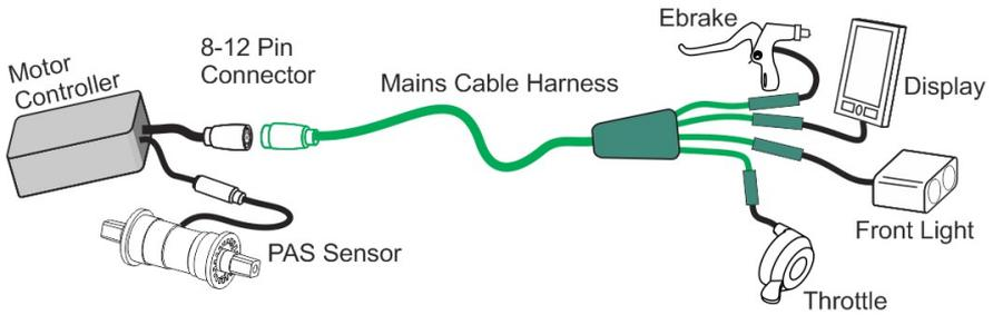
**Figure 1: Example of a Mains Harness (Green)**
