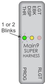
On releasing the lever, the green LED will blink in a flash pattern to indicate the selected control mode:
