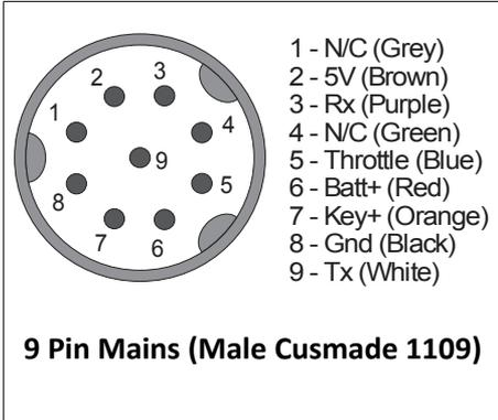
The 9 pin main hookup to the Phaserunner or Baserunner controller uses a male Cusmade 1109 connector. The Tx and Rx lines pass through to the display.
