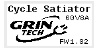
Figure 2: Splash Screen after power applied, shows Model and Firmware Version
