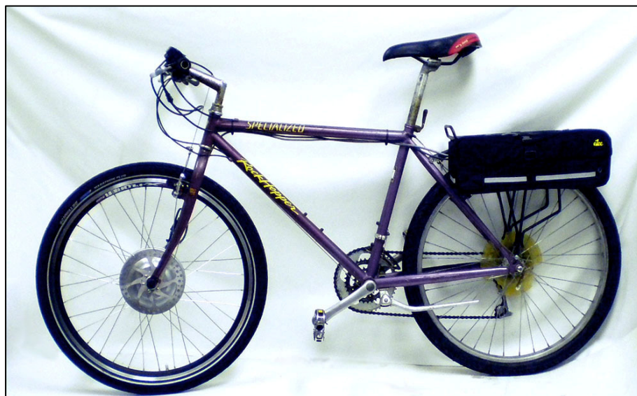
New eZee Kit installed on an old purple mountain bike
