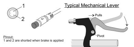
This is the Pull version, suited to mechanical brake levers and some hydraulics. A push version is also available for levers with a different pivot geometry.
