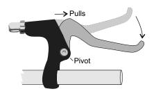
This is the Pull version, suited to mechanical brake levers and some hydraulics. A push version is also available for levers with a different pivot geometry.
