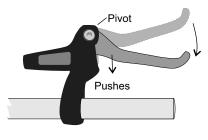
This is the Push version, suited to most hydraulic brake levers. A pull version is also available for levers with a different pivot geometry.
