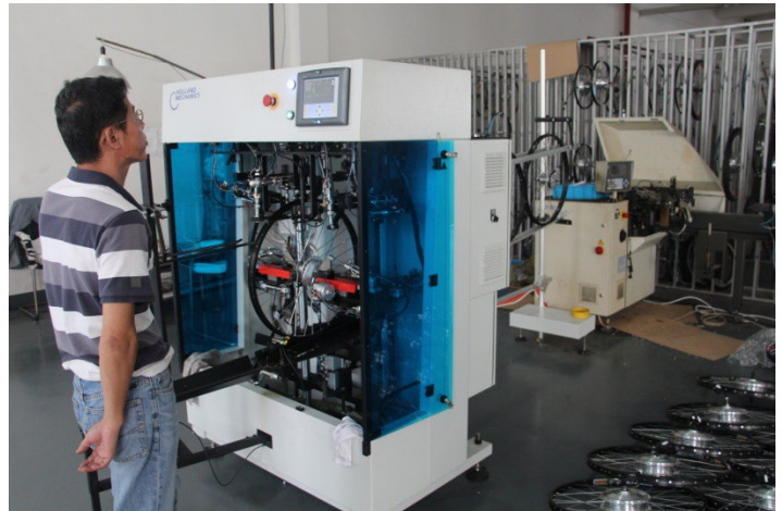
Automated wheel building Holland Mechanic M/C
