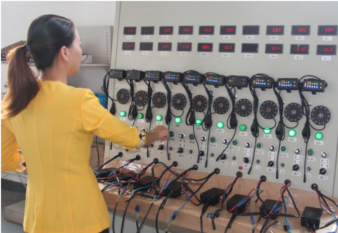
Ageing test on controllers, 100 % tested
