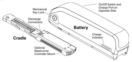
The cradle is designed for mounting to waterbottle eyelets on the bike frame using M5 screws, but can be installed more securely and with greater versatility using Grin's *Triple Bob* battery anchor. The pack slides in and out of the cradle for easy removal to charge indoors, with a key and barrel lock to hold it secure.
