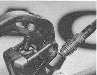
If possible cut the line about 10cm/4" away from the master cylinder. Use an 8mm open end spanner and take out the sleeve nut and pull out the line.
