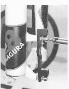
Assemble the calliper to frame/fork after installing the wheel with the rotor.
