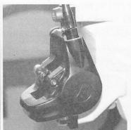
Take a Torx T25 key and unscrew the bolt which holds the line by opening 30° counterclockwise. Now you can turn and adjust the angle of the line as required. When adjusted, tighten bolt with **3Nm**.
