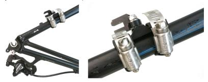
Place the motor into the rear dropouts and line up the hole in the torque arm with the slot in the frame clamp.
