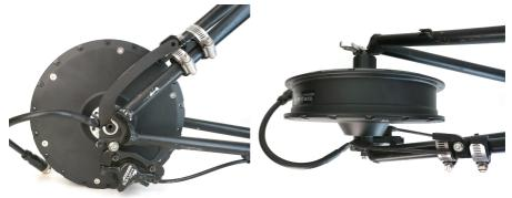
Insert and loosely secure the motor with the quick release skewer. The lever of the quick release skewer should be on the torque arm side. Verify that the torque arm is fully seated in the motor.
