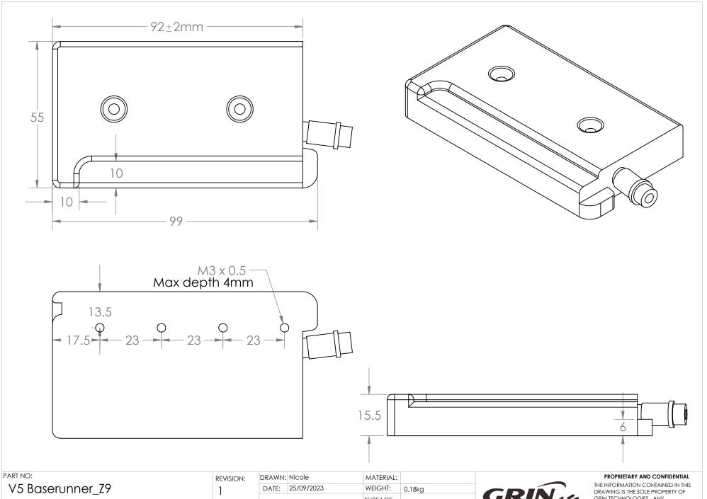
**DESCRIPTION:** 36-52V Field Oriented Motor Controller UNLESS OTHERWISE SPECIFIED: DIMENSIONS IN MM TOLERANCES ±0.5mm TWO PLACE DECIMAL ±
