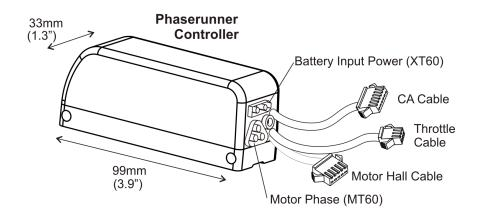
However, unlike standard trapezoidal or sinewave controllers, the Field Oriented Controller (FOC) needs to be tuned to the specific motor that it is paired with. For that you need the USB->TTL communication cable and a computer with the Phaserunner software suite installed. You cannot just connect the phase and hall wires to a random motor and expect it to run.
