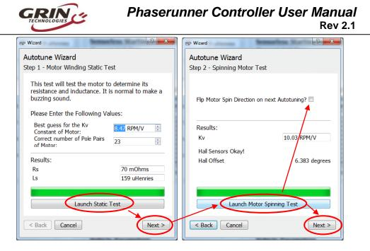
During this spinning test, the Phaserunner will be self starting the motor in sensorless mode. If the motor fails to spin and just starts and stutters a few times, then you will need to adjust the sensorless starting parameters as described in section 4.4 until the motor is able to self start OK.
