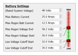
With the controller mapped to your motor and spinning fine, you should next set the battery voltage and current settings to appropriate values for your pack. We recommend making the max regen voltage the same as the full charge voltage of your battery, with the regen start voltage about 0.5V less. For the low voltage rollback, you can set this to be just above the BMS
