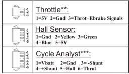
\*\* Ebrake / Throttle wires can be separated if desired
