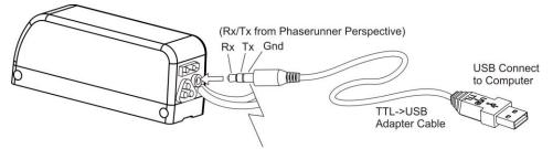
The communication standard uses a 5V TTL level serial bus, and Grin produces a 3m long TTL->USB adapter cable so that you can connect with the USB port of a standard computer. This is the same communication cable used with the Cycle Analyst and Satiator products. You can also use 3rd party USB->Serial cables, such as FTDI's part number TTL-232R-5V-AJ.
