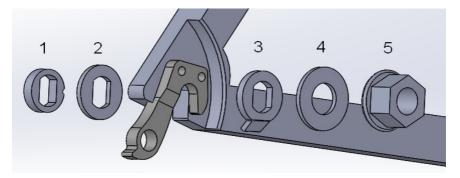
If using a torque arm, mount it on this side between the outside of the dropout and the large washer. The tabbed washer can be omitted if using a torque arm.
