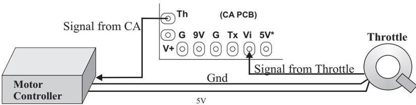
In this manner, if full throttle is set to be 20 amps, then by riding half throttle, you could ensure exactly 10 amps are drawn from the battery regardless of the vehicle speed, giving the user more direct control over their power usage. Similar setups can be used to implement accurate cruise control systems.
