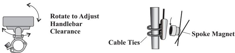
In the case of the CA-SA, CA-DPS, and CA-HC models, there is also a speedometer pickup cable and spoke magnet. The pickup attaches to the fork with two cable ties, and must be mounted to pass within 2mm of the magnet for the speed readings to register. For systems like scooters or motorcycles that don't have spoked rims, a standard magnet can be attached with epoxy to a suitable location on the wheel.
