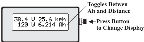
A quick press of the button will show other display screens of interest, while holding the button will reset trip statistics. The second display shows just the electrical information of the battery pack, including the current in amps.
