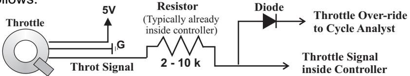
There are various setup options which control the speed at which the Cycle Analyst responds to these signals. If the settings are too fast, then the control can be twitchy or oscillate around the desired value, while gain settings that are too low will cause a long lag time before the limiting kicks in.
