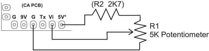
The optional resistor R2 is used to reduce the potentiometer wiper range from 0-5V to just 0-3V so that the entire turn range is utilized. In the advanced setup menu, you can select whether this voltage regulates the current limit or the speed limit, and it will scale the limit between 0 and the speed/current limit programmed in the setup menu.
