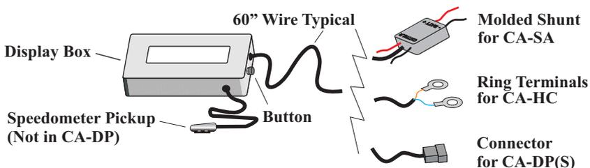
The Cycle Analyst picks up the vehicle speed information using either a spoke magnet, or in the case of the CA-DP device, through the hall sensor signals from a brushless motor controller.
