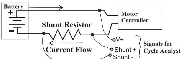
This shunt resistor must be wired in series with the negative lead of the battery pack. The power to run the Cycle Analyst then comes from the connection to the positive lead of the battery.
