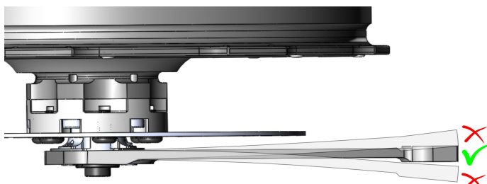
Figure 10: Torque Arm must not be flexed in or out
