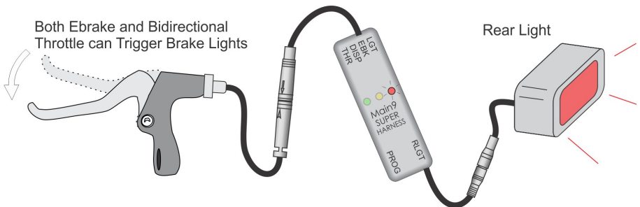
Figure 12: The rear light port can be used as a brake indicator in modes 3, 4, and 5.
