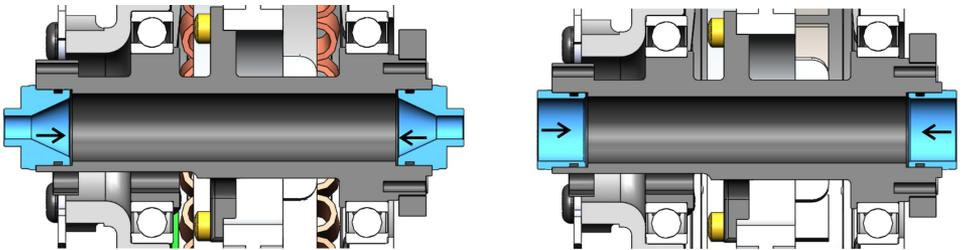
**Figure 7: Example of quick release (left) and thru-axle (right) end caps, slid into place.** In most adapter kits the left and right caps are identical.
