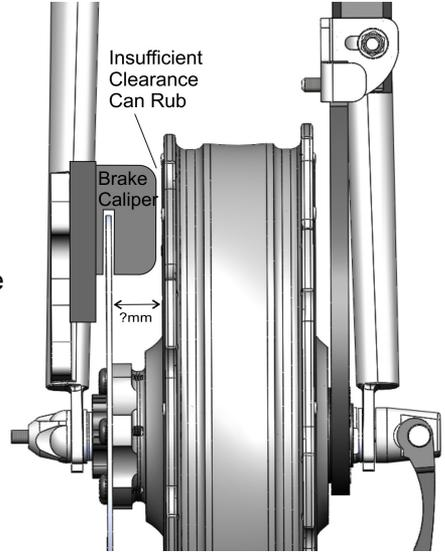
Figure 13: Illustration of Caliper Clearance.
