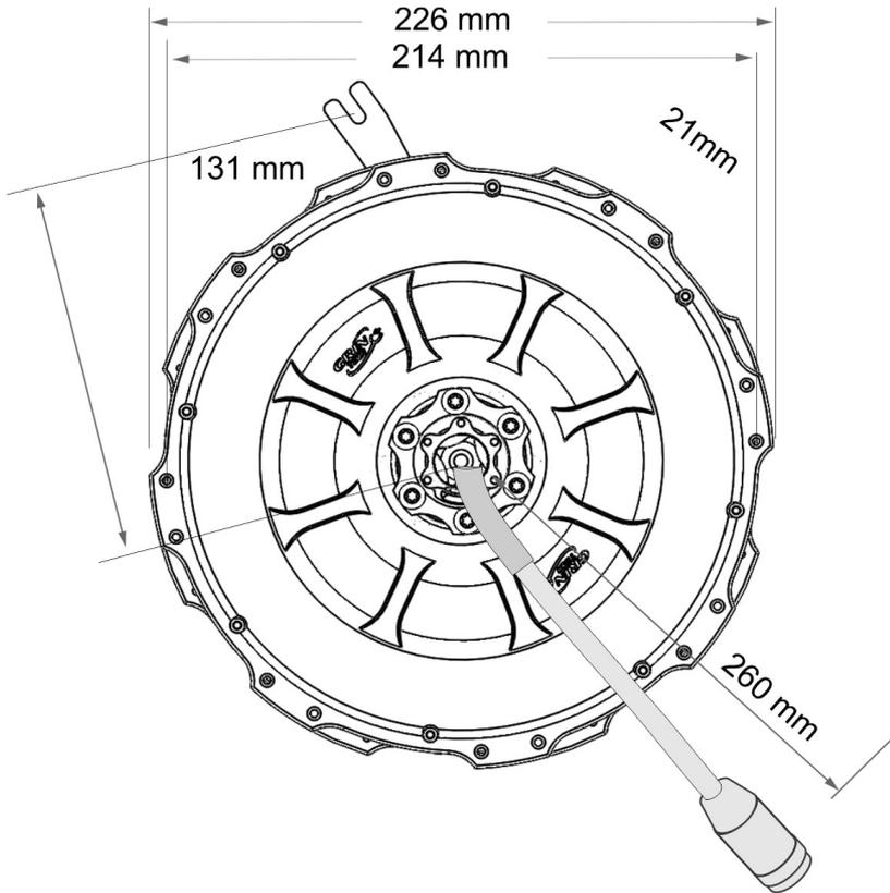
Figure 15: Mechanical Drawing
