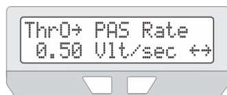
Example setup with fast throttle response and more gradual power engagement from pedal sensor
