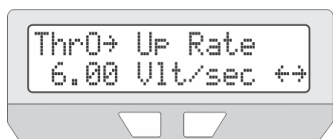
Example setup with fast throttle response and more gradual power engagement from pedal sensor
