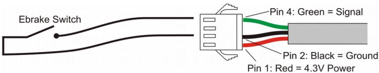
**Figure 12: eBrake Connector. 5V+ for Hall Brakes**
