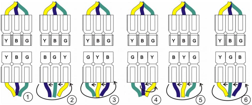
**Figure 9: Systematic Approach to Phase Pinout Mapping**
