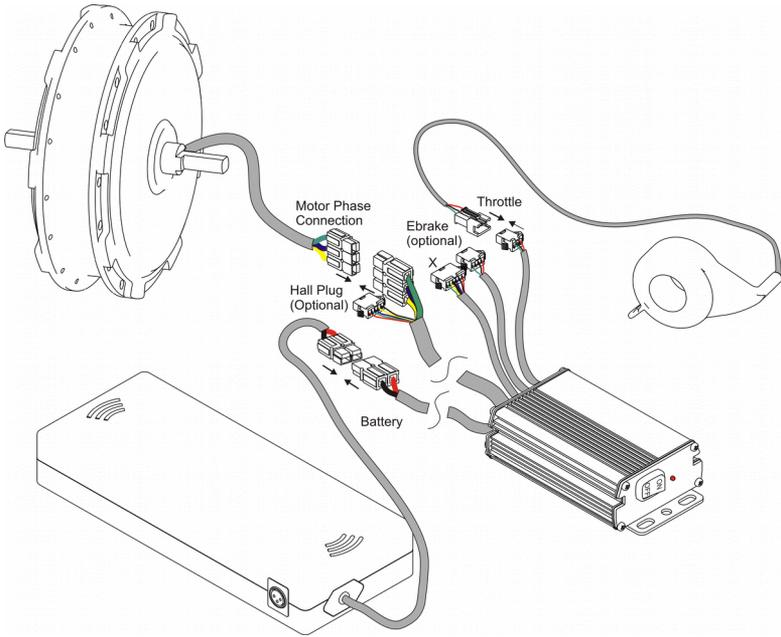
**Figure 3: Basic hookup diagram (motor, throttle, and battery)**
