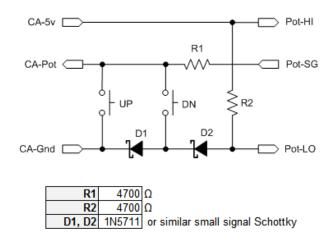
The circuit above might be constructed as an in-line adapter as shown here, wired inside the switch housing, or attached directly to the CA PCB AuxPot pads with short AuxA and AuxD wiring running out of the case back to JST connectors.
