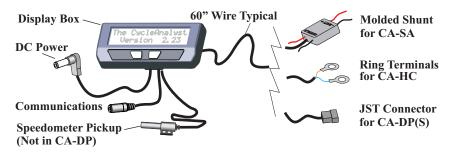
The Cycle Analyst picks up the vehicle speed information using either a spoke magnet, or in the case of the CA-DP device, through the hall sensor signals from a brushless motor controller.
