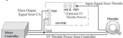
In this manner, if full throttle is set to be 20 amps, then by riding half throttle, you could ensure exactly 10 amps are drawn from the battery regardless of the vehicle speed, giving the user more direct control over their power usage. Similar setups can be used to implement accurate speed control systems. Note that it is essential to set the AuxVoltage input (see 8.17) to either the current or speed limit first, otherwise the system will take off at full power when turned on.
