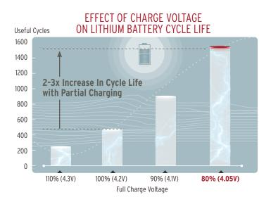
With the Cycle Satiator, you can program your primary profile to give an 80% charge, and have a secondary profile that does a 100% charge when you need full range. Then have the best of both worlds, a battery that lasts thousands of cycles but still goes the distance when you need it.
