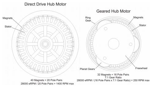
Figure 16: Direct Drive and Geared Hub Motor eRPM examples
