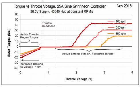
Figure 13: Regen intensity for throttle 0V-0.8V
