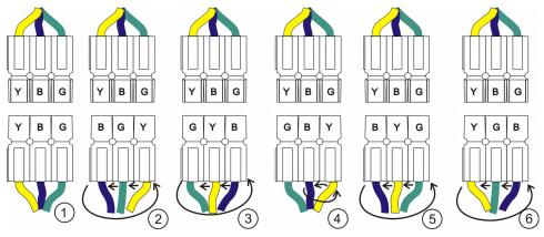
Figure 9: Systematic Approach to Phase Pinout Mapping
