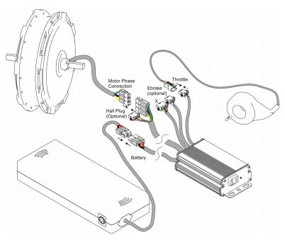
Figure 3: Basic hookup diagram (motor, throttle, and battery)
