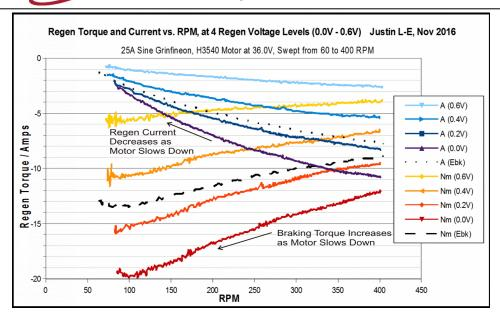
Figure 14: Regenerative Braking Torque and Current as a Function of Motor RPM at 4 different throttle regen voltages and also with ebrake lever pressed (Ebk, dashed lines)
