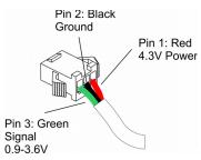
**Figure 4: Controller Throttle Pinout**
