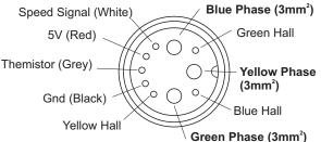
\* Pin-colour combinations are intentionally different from Higo pin-colour standard
