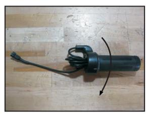
You should see the voltage rise until it reaches about 4V. This means the throttle is operating correctly.
