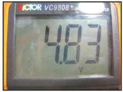
Next test the throttle signal by placing the probes between the black (ground) and the green (signal). Note that sometimes the signal will be a white wire.
