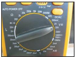
Switch the multimeter to DC voltage mode and turn the dial to the "20V" setting
