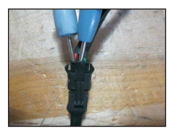
You should see somewhere from 4V to 5V. With this series of tests it doesn't matter which way round the probes go - the only difference is that you'll see a negative voltage if you reverse the them. If you have issues getting the probes to fit in the back of the housing then you can try putting a small pin or nail in first and then use the probe on that.
