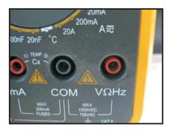
Make sure your multimeter has the black probe in the COM slot and the red probe in the  $V\Omega Hz$  slot.
